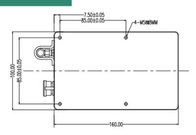
Unit size without antenna = 160mm x 100mm x 83.2mm
